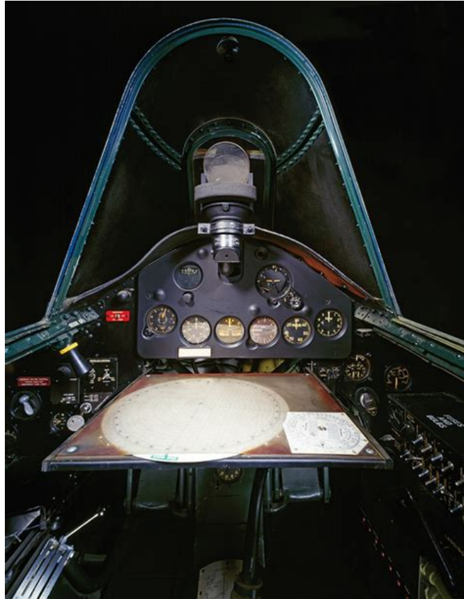
Fig 1. A Mk. 3A plotting board installed in an aircraft.
